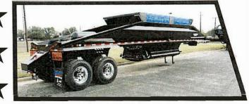
Renegade Trailers mission is to provide our customers with the most high quality belly dumps on the market. With a 30 yard capacity, extremely durable yet lightweight frame, and load pinching ability, we strive to provide our customers with the best possible equipment for the job at hand.
